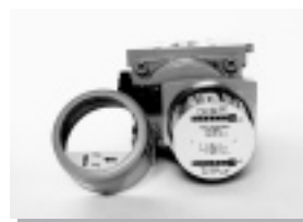
Index with its rotatable cover removed, showing the dual indexes.
